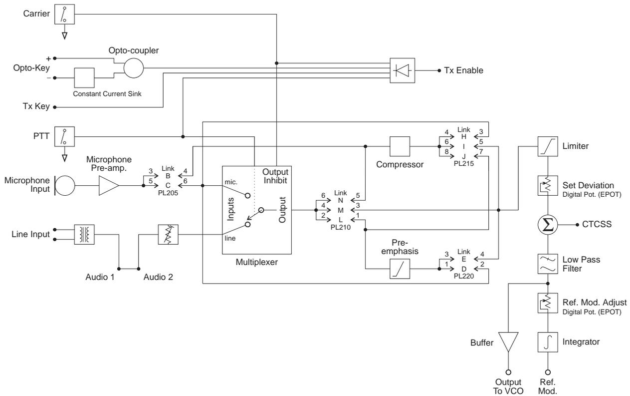
Figure 2.6 T826/827 Audio Processor Block Diagram
