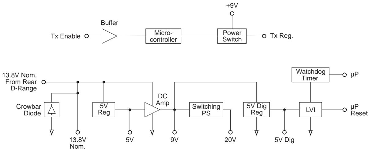
**Figure 2.7 T826/827 Power Supply & Regulators Block Diagram**
