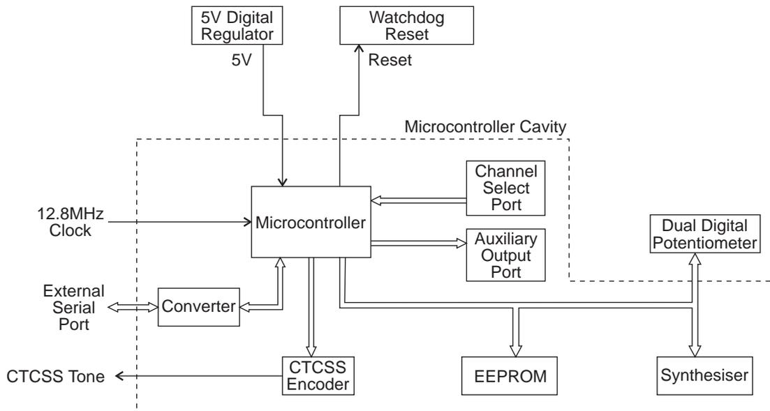
**Figure 2.3 T826/827 Microcontroller Block Diagram**
