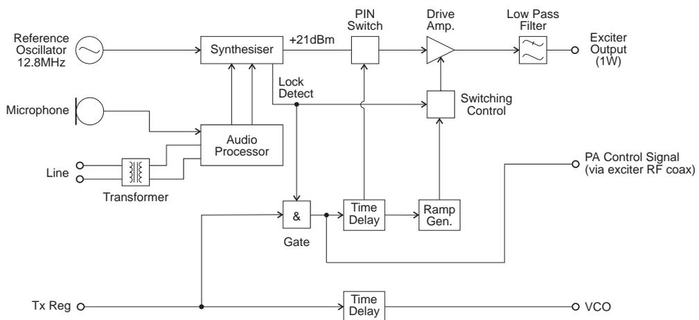
**Figure 2.2 T827 High Level Block Diagram**
